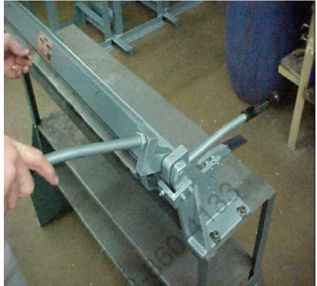
5. Return the bending lever to its original position at the rear of the machine. Place the partially formed part against the nose of the bending blade. Pull the bending beam lever toward you while holding the work material in the machine until the blade contacts the part. Push the lever down to finish forming the flange.
