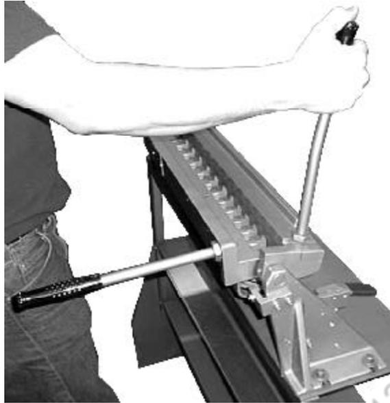
7. As you lift up on the lower beam lever the work piece will exit on the back side of the machine.
