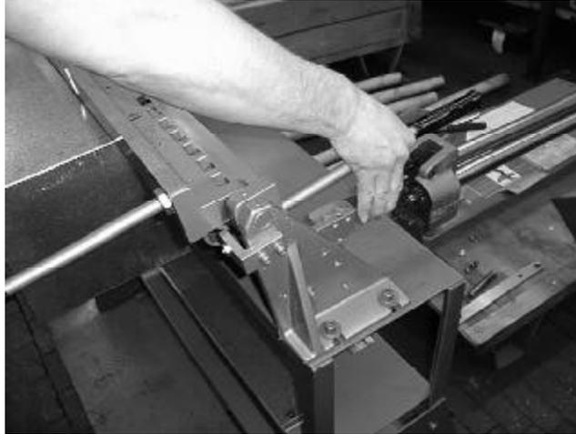
3. Grasp the lower beam lever and, with the last finger or two of your hand, pull up on the lower beam release until the part is released from the bending blade.
