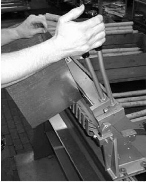
5. While you hold onto the work piece, return both of the beam levers to their starting position. Allow the work piece to rotate with the beams while supporting it with your free hand. The duct will slide free of the bending blade as the levers approach vertical.
