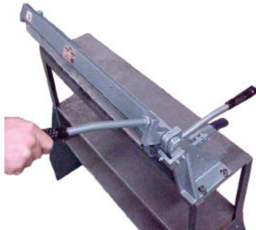
4. Pull the bending beam lever toward you until it stops.
