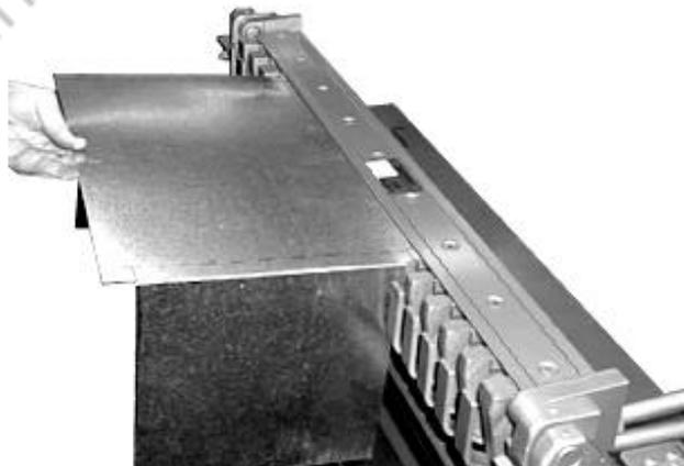
2. Make sure that the work piece is inserted under the bending blade as far as it will go. Pull the bending beam lever toward you until it stops.
